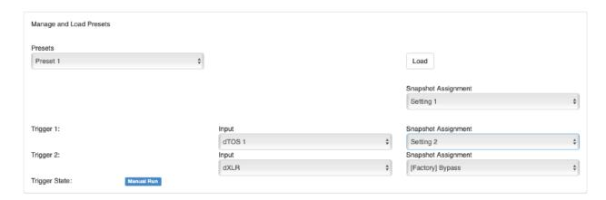
In a second step, the stored snapshot is assigned to a preset and/or a trigger.
